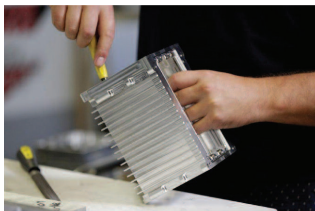
Solent Manufacturing in action: Aluminium enclosure deburred by hand at Innova Design and Build
